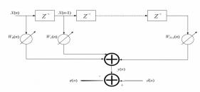
Fig. 2. N-tap transversal adaptive filter.
